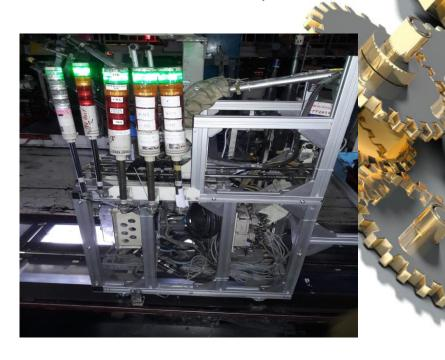
Maruti Suzuki, Manesar – Washing Station addition in JGC gear inspection machine (13 sets)
